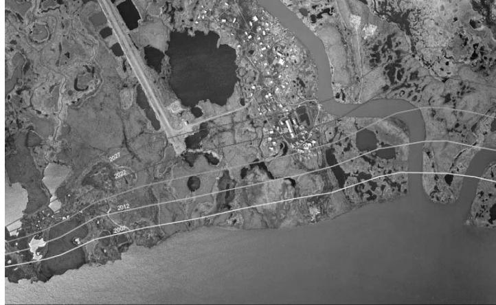
Alaska District Corps of Engineers Civil Works Branch Predicted and Historical Shorelines 2007 2012 2017 2022 2027 0 250 500 750 1,000 Feet 1 INCH EQUALS 500 FEET IMAGE DATE: JULY 2024 Alaska Village Erosion Technical Assistance Program Newtok, Alaska
